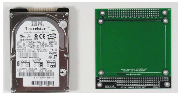
DK-LINUX-HD10 10GB hard drive (left) with full Linux pre-installed; includes hard drive mounting board (right) and cable.
